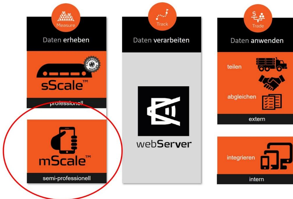
mScale manually records data that is measured or collected digitally and performs calculations in terms of volume and more. The GPS function of the mobile device documents the location. Based on colour panorama photographs taken by the user, the number of logs can be determined using photo-optical means. A sampling of diameters makes it possible to derive a distribution of diameters for piles.
