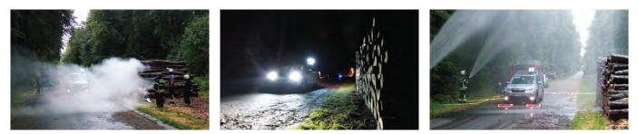
sScale<sup>™</sup> has a maximum error of +/- 3% relative to traceable reference areas on real woodpiles. Fixed outer contours of woodpile face areas are measured regardless of device user or sScale<sup>™</sup> system under all test conditions with a maximum deviation of +/- 3%, based on the average value.
