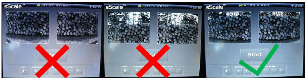
Figure 4: Too low, too high and correct camera alignment
