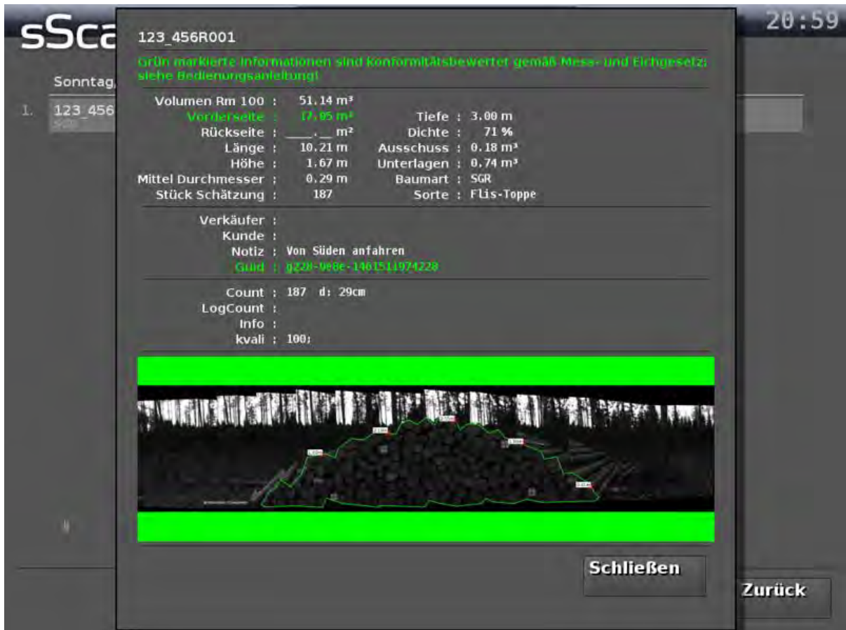
Figure 21: Result representation of a conformity-rated measurement in the user interface "Details of an archive entry"
