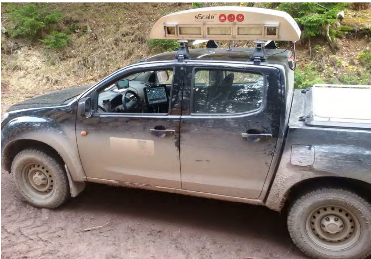
Figure 1: Example of a sScale™, carrier vehicle with rooftop camera unit and touchscreen in the passenger area
